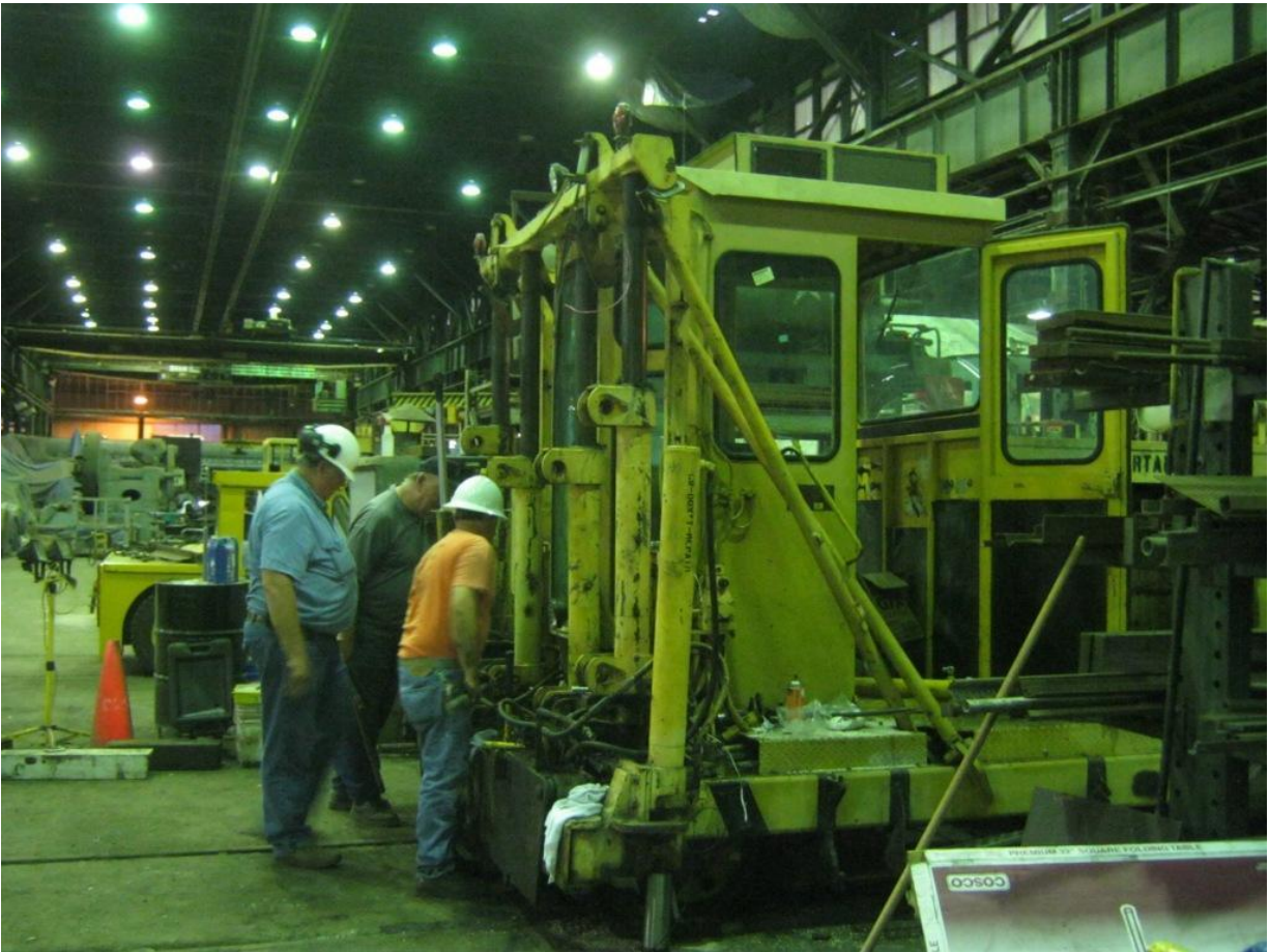
Chris, Gene, and Mike H. reassemble the slide columns on the “new old” tamper
